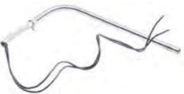
RFHE5 OCEAN 'L' SHAPE ELEMENT - 220V 260W - 9,5mm O.D. 190mm long (total)
