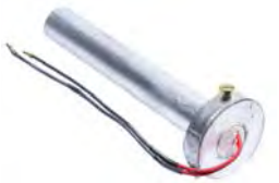
RFHE4 OZEN FREEZER ELEMENT - 220V 350W - 25mm O.D., 185mm long with mounting piece
