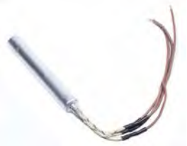
RFHE2 CARAVAN FRIDGE/FREEZER ELEMENT - 12V/220V 115W - 17mm O.D. 121mm long
