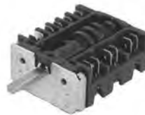
SW500 7 POSITION ROTARY SWITCH 6 heat + off, suitable with DEFY, KELVINATOR, KIC and other solid plate hobs type: EGO 46.27266.500
