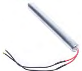
RFHE8 ELECTROLUX FREEZER ELEMENT - 220V 220W - 21,4mm O.D. 195mm LONG
