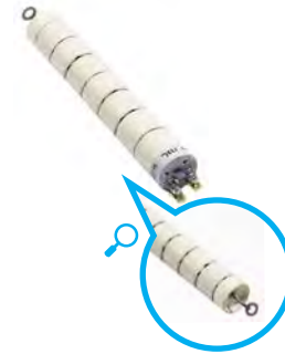
RFHE3 BARLOWS CERAMIC ELEMENT - 220V 400W - 29,6mm O.D. 170mm LONG
